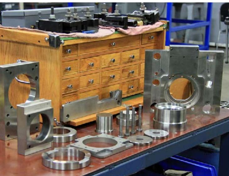
*Die components are engineered for full interchangeability and manufactured to exacting tolerances.*
